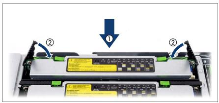
Figure 37: Installing a memory board
